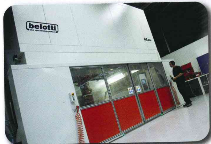
► New machinery from Belotti has added large capacity 5-axis milling
