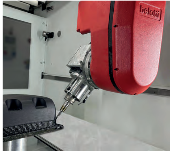
→ The BEAD machine milling a thermoforming mould (above)
